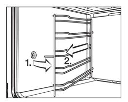
■ Pull the runners forwards out of the holder and remove.
